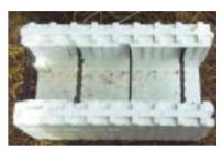
Figure 2: The 250mm-thick 'standard' blocks with PE ties.
